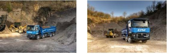
With payload capacities edging up close to 20 tonnes says Scott, the 32-tonne Thompsons muck-away day-cab Range C 430.32 N3Gs currently available are powered by 11-litre 430hp/2050Nm engines. They are married to 12-speed Optidriver automated gearboxes. Fitted with single hub reduction axles and Optibrake engine brake/retarders, the trucks are shod with Bridgestone 315/80 R22.5 tyres.
