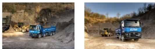
With payload capacities edging up close to 20 tonnes says Scott, the 32-tonne Thompsons muck-away day-cab Range C 430.32 N3Gs currently available are powered by 11-litre 430hp/2050Nm engines. They are married to 12-speed Optidriver automated gearboxes. Fitted with single hub reduction axles and Optibrake engine brake/retarders, the trucks are shod with Bridgestone 315/80 R22.5 tyres.
